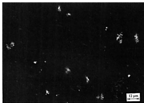
Figure 8 Crossed polarizing micrograph of 10GTS-AGlyd crosslinked with Resimene 746 at room temperature.
